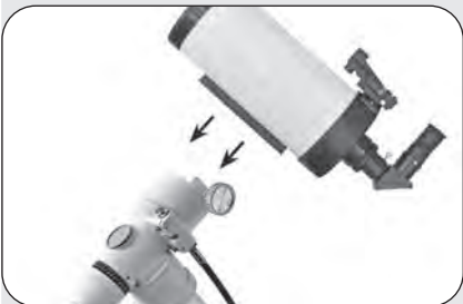
Fig. 8a: Inserting the optical tube with the prism rail into the prism holder and fixing it in place.
