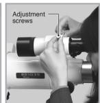
3 While looking through the finder scope, align the field of view with the telescope's field of view by loosening or tightening the adjustment screws on the finder bracket so that the target comes close to the center of the field of view.
