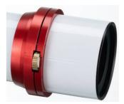
The Etalon of the LS40THa is tilted rather quickly as you turn the wheel. Therefore, turn this wheel very slowly to avoid missing the optimal tuning point.
