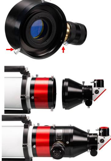
Install the telescope now again on your mount, and point it to the sun. Move the handle of the originally Pressure-Tuner back into the position which you have previously noticed.
