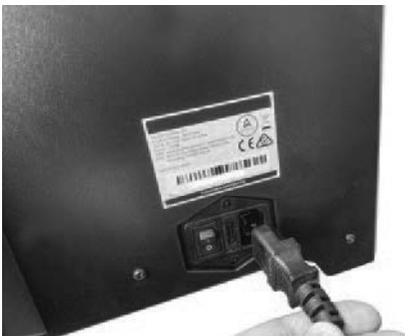
1. Take the power cable and plug it into the printer's power input.
