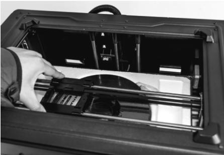
9. Slide the X-axis guide rail to the very back by hand.
