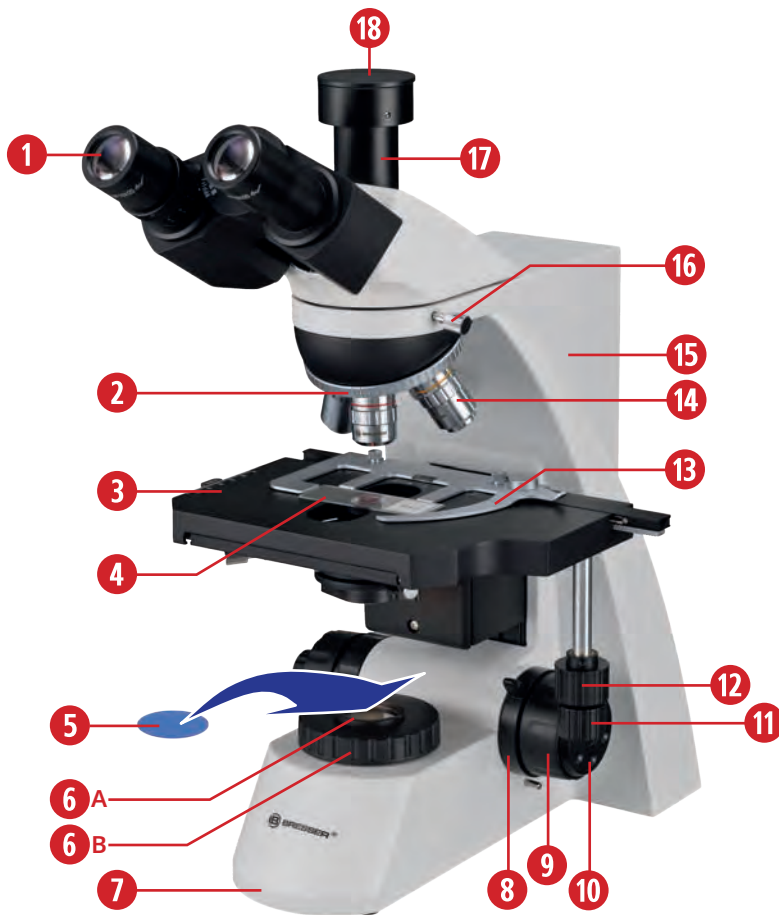
Fig. 1A: Components on TRM 301, front/side view.
