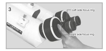
2 Attach the eyepieces so that the chrome barrel of the eyepiece is push into the eyepiece holder entirely. When you exchange the eyepieces, you should align the optical axis of left side and right side eyepieces in the procedure stated in ALIGNMENT.
