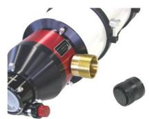
At the front of the black handle you will find a small cover cap with the label "Lunt Solar Doppler True Tuning". Unscrew this cover cap. Behind the cover cap you will find a screw, remove this screw by using the hexagon wrench that is delivered with the PC-USB controller. Now you can
