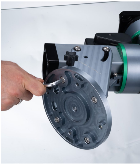
Remove one of the two lateral bracket
